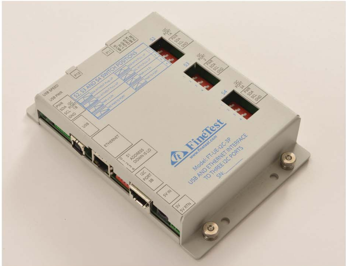
USB or Ethernet to 3 I2C Ports Communications Adapter
