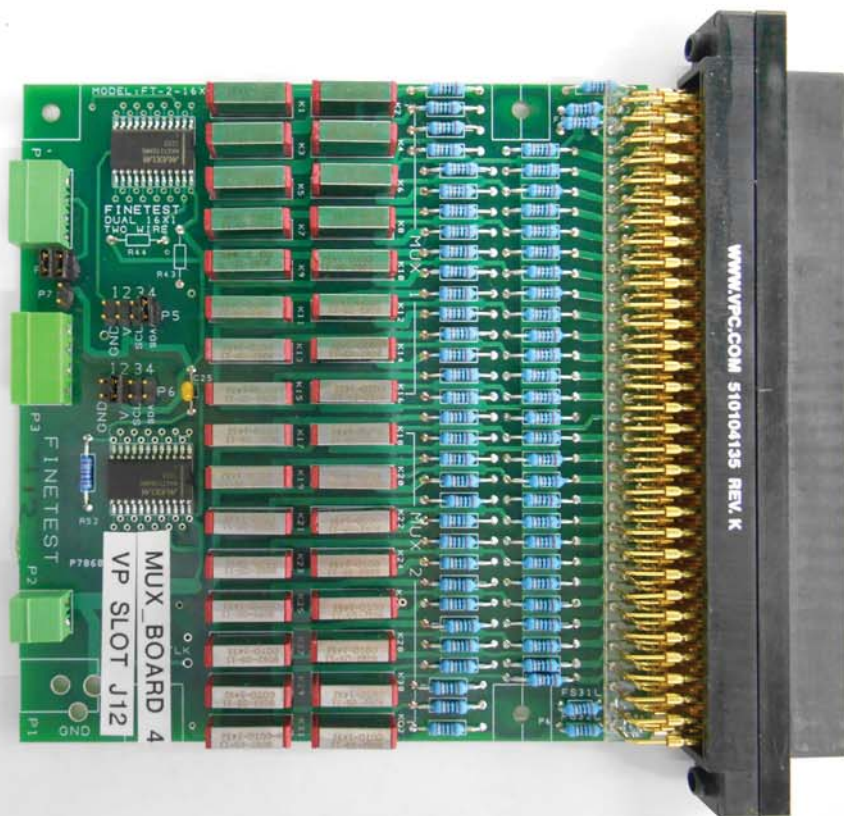
Dual 16 x 1 Mux Card with cover removed
