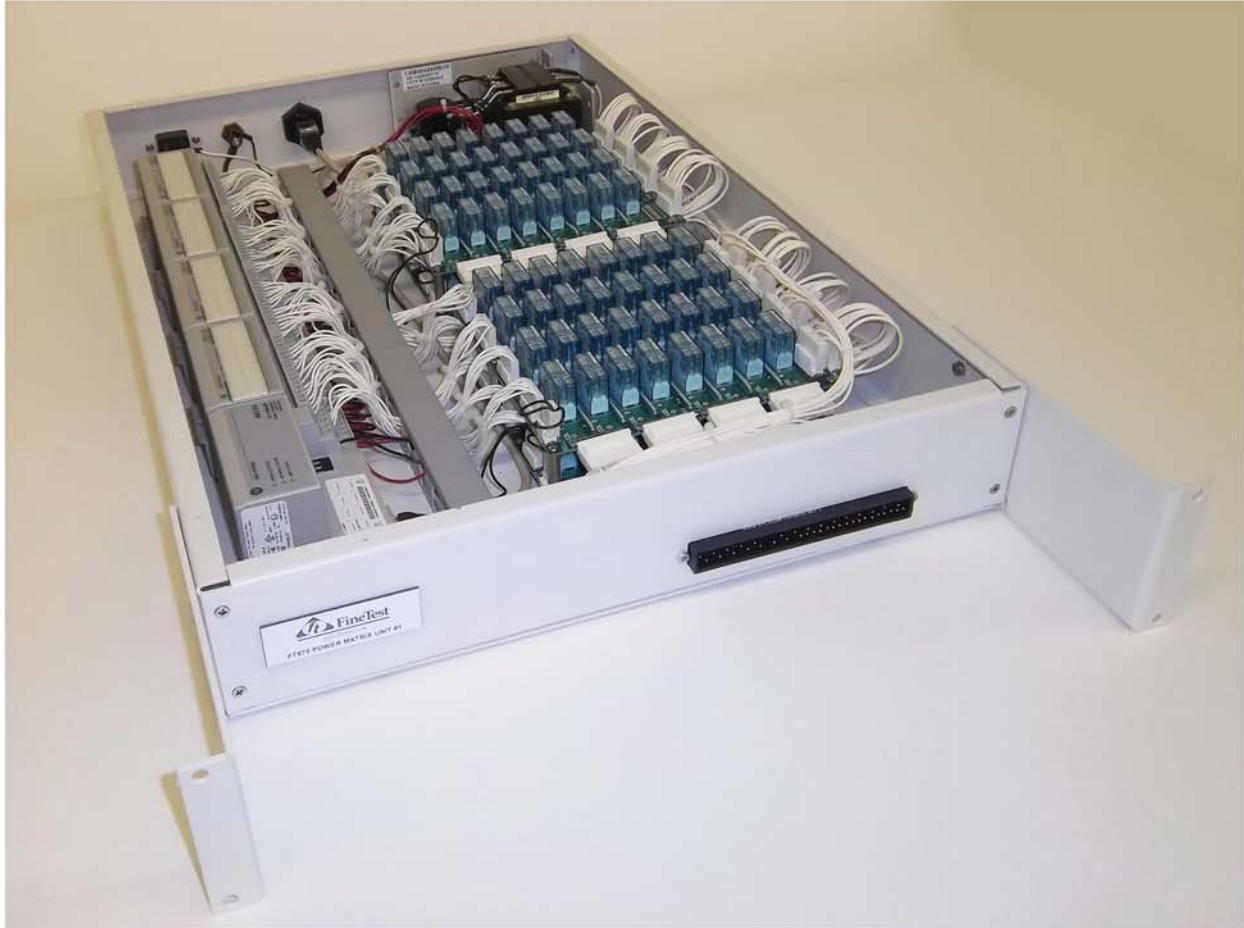
Top Angle view of Power Matrix Unit
